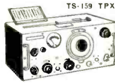
Measures frequency between 150 & 200 mc. by heterodyne method. Power of Xmr. can be directly measured. Measures DC voltages up to 500 Volts. Original operation on 110 V. 400 cy. but conversion kit makes it operable on 110 V. 60 cy. New, complete with tubes, crystal, cal. chart, antenna, meter & conversion kit and data for 110 V. 60 cy operation $29.95
